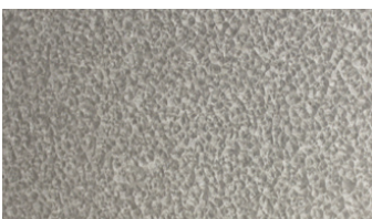
55% Al-Zn Alloy Coated Steel with Acrylic Coating (97)
